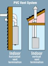
All indoor tankless units must be vented vertically or horizontally to the outdoors using manufacturer approved venting material. See the installation instructions for each specific model. (ULCS636 Pipe must be used for Canada.)
